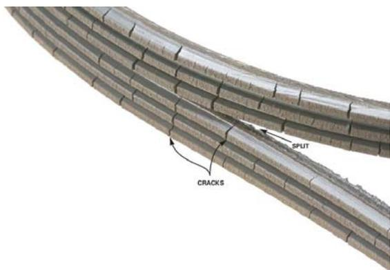
Hoses should feel firm, not mushy, be free of obvious cracks and show no evidence of leaking at connections. Belts shouldn't be cracked, frayed, brittle or glazed looking and should be firmly, but not too tightly tensioned.
